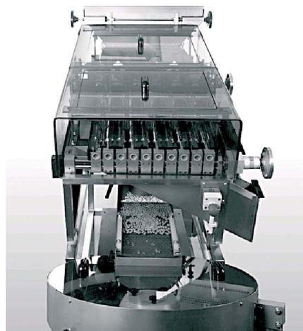
L 650 in combination with a Seidenader DS thickness sorter: The products are sorted by thickness and length.
