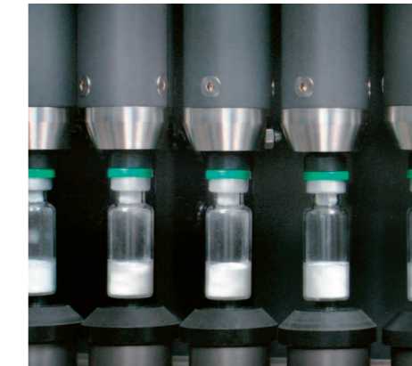
HSA unit integrated in inspection machine Seidenader MS
