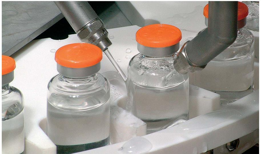
Dry caps, seals and crimps through exact adjustment of the water nozzles
