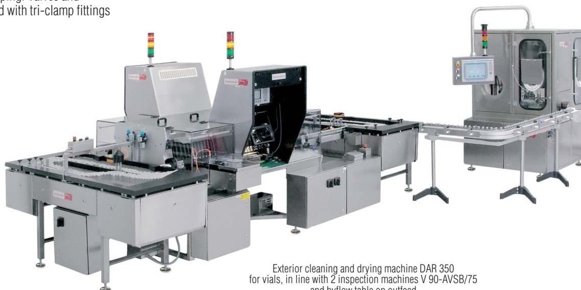
Exterior cleaning and drying machine DAR 350 for vials, in line with 2 inspection machines V 90-AVSB/75 and byflow table on outfeed
