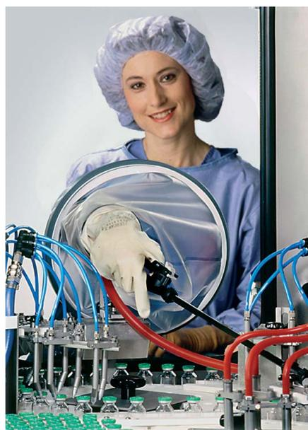
DAR with optional isolation system and glove parts for toxic products
