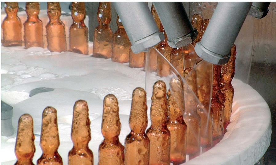
Cleaning nozzles with graduations for precise adjustment, reproducible for each format.
