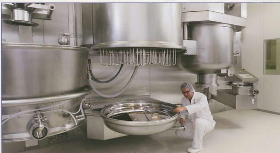
Inspection of fluid bed system after cleaning
