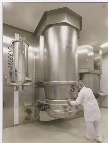
Check of granulation process through inspection window
