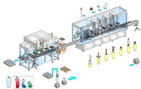
The flexible, linear modular design enables conversion for a different product in just a few minutes.
