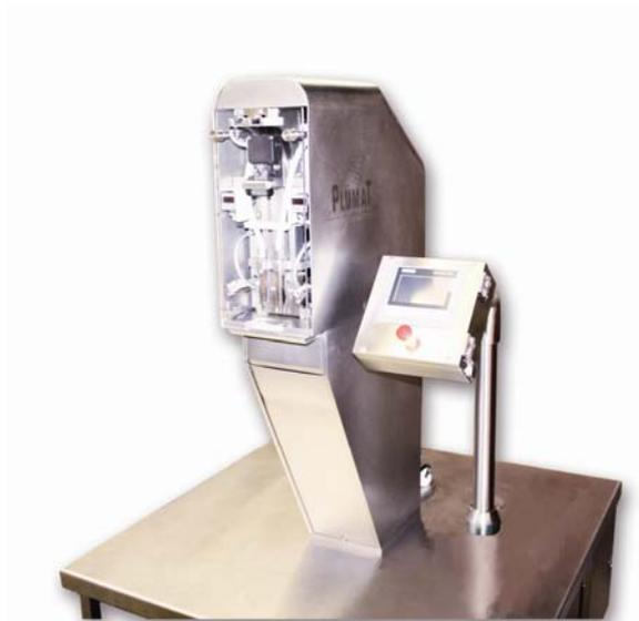
The **Plümatex-BFM 007-SFC** Filling and Sealing Machine was designed as a table-top device to process the bags with SFC-System (Single-Function-Connector), which was developed and patented by Plümat. Bag as well as Sealing Caps will be manually fed into the machine. All further operations are running automatically.
