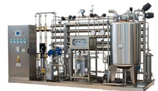
**Thermocompressor with new compressor side channel blower and Clean Steam**
