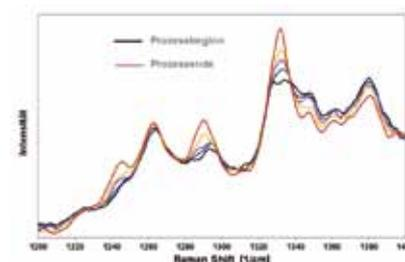
Fig. 3: Raman spectra of tablets during coating
