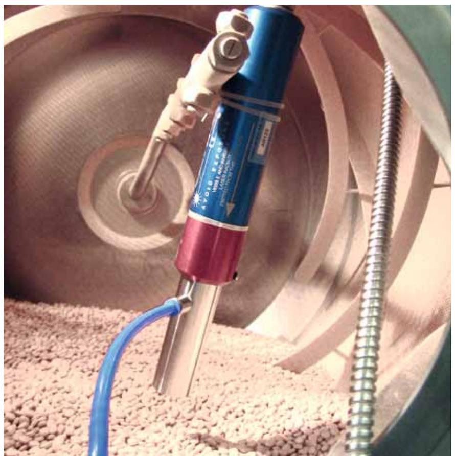
Fig. 2: BFC 50 TriPan with integrated PhAT probe
