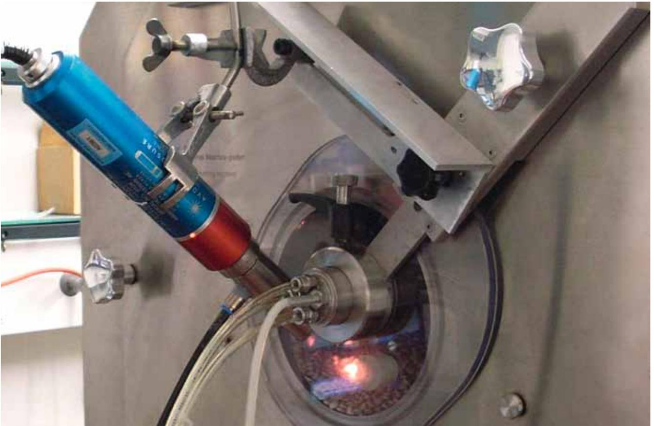
Fig. 1: BFC 5 lab coater with integrated PhAT probe
