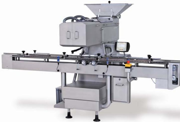
**CF-1220:** 12-channel high-speed tablet and capsule counter with single-track bottle conveyor.
