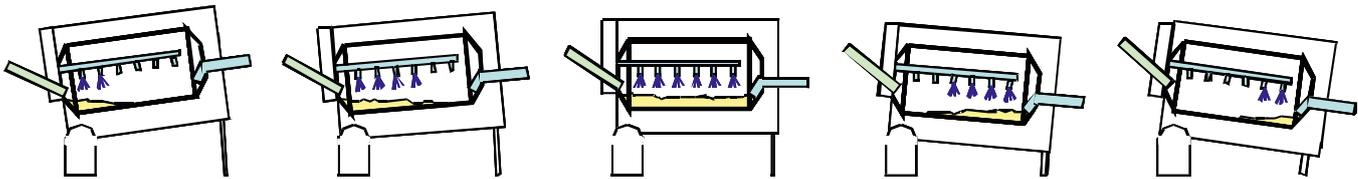
To complete the continuous coating cycle, the process is reversed by tilting the pan into a negative inclination while shutting down spray nozzles group by group as coated tablets are discharged. Mounting or dismantling the individual spray guns from the support arm is simple
