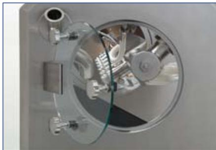
vidual return flow assembly for recirculation of the suspension flow. This feature allows the coating suspension to stay in flow during the beginning or towards the end of the continuous process to avoid sedimentation during spray interruptions. Each nozzle group can be controlled individually to precisely adjust the required spray rate.
