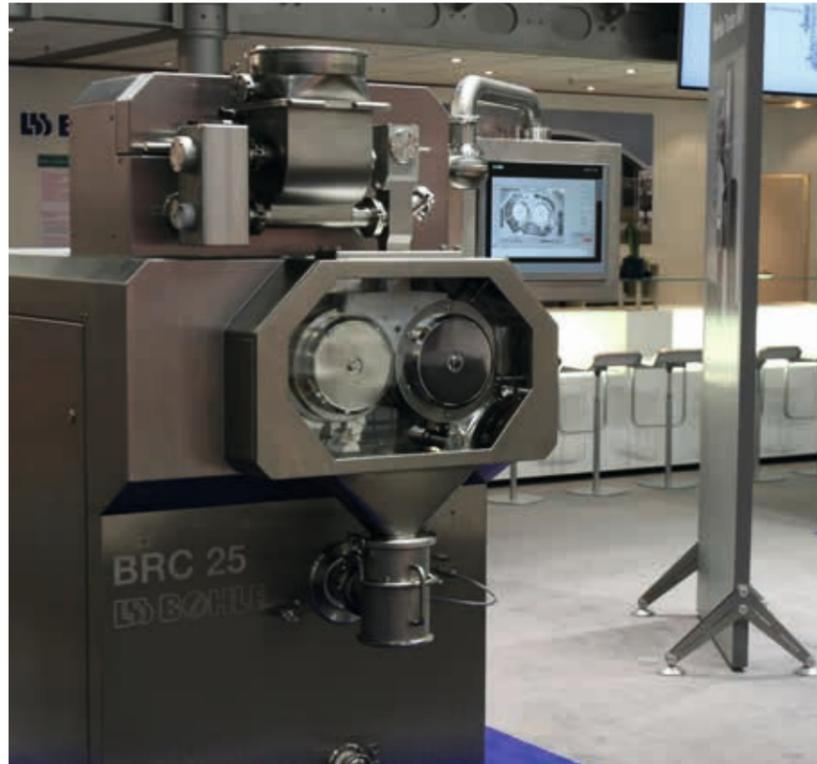
tion to make the scale-up of BRC 25 to BRC 100 as easy as possible. This is ensured through the identical roller geometry and control in both machines.
